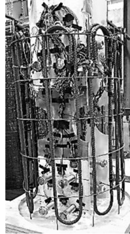
(b) (c) Figure 2.3 Longitudinal reinforcement in the repair region: (a) closed bar profile, (b) distributions of rebars, and (c) reinforcement cage
